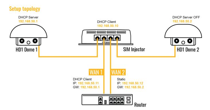
In this scenario, each HD Dome creates a WAN connection to the main router. A single SIM Injector is used to provide SIM cards for each HD Dome. The HD Dome can be replaced with any Peplink cellular router supporting RemoteSIM technology.
