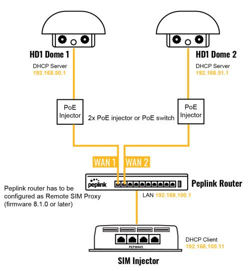
In this scenario, SIMs are provided to the HD Domes via the main router. In this example, the **Remote SIM Proxy** functionality needs to be enabled on the main router.
